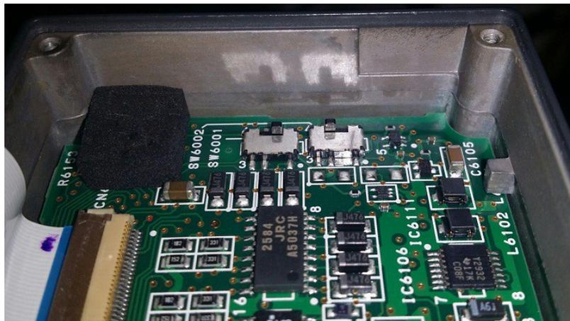
Figure D3: Hitachi KP-FD30 internal switch setting for external trig/shutter mode.
