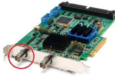
Figure 2: Karbon-CXP2 rear ports
